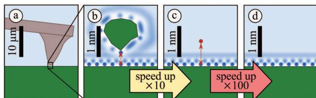
FIG. 1. Simplifying the model system, reducing the computational effort by several orders of magnitude: (a) The actual experimental setup, inaccessible to atomistic simulations; (b) free energy calculations with a fully solvated nanocluster tip; (c) free energy calculations with a single water molecule as tip model; (d) local water density calculation from equilibrium simulations.
