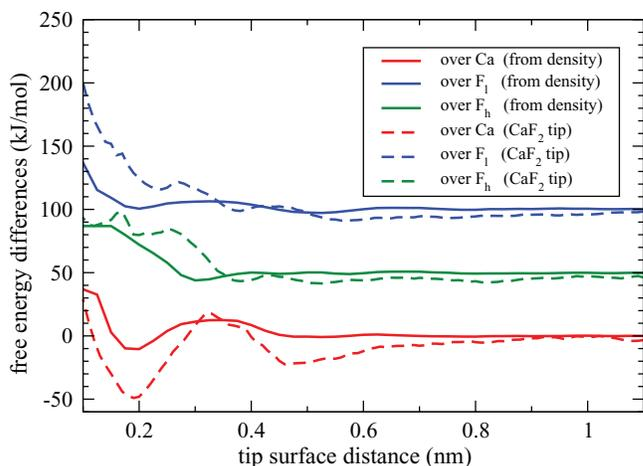
FIG. 5. Comparison of the simple model and simulations with an explicit nanocluster tip: Free energy curves over Ca (red), Fh (green), and Fl sites (blue) in a fluorite surface. Curves obtained from the local water density are solid, curves obtained from FEP with a sharp  $\text{CaF}_2$  nanocluster tip are dashed.
