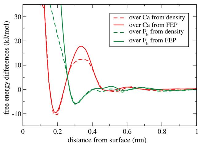
FIG. 4. Comparison of the free energy curves for water molecules above  $\text{CaF}_2$  with those obtained from the water density using Eq. (1). Density derived curves are dashed, and those from free energy perturbation calculations are shown as solid curves.
