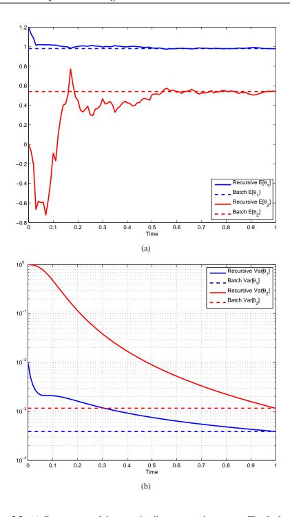
**Figure 2.3:** (a) Convergence of the recursive linear regression means. The final value is exactly the same as that was obtained with batch linear regression. Note that time has been scaled to at k=K. (b) Convergence of the variances plotted on logarithmic scale. As can be seen, every measurement brings more information and the uncertainty decreases monotonically. The final values are the same as the variances obtained from the batch solution.
