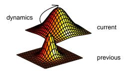
**Figure 3.1:** Visualization of the prediction step: the prediction propagates the state distribution of the previous measurement step through the dynamic model such that the uncertainties (stochastic terms) in the dynamic model are taken into account.
