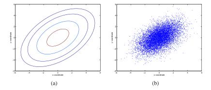
**Figure 3.8:** (a) Two dimensional Gaussian density. (b) Monte Carlo representation of the same Gaussian density.
