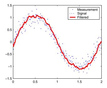
**Figure 2.5:** Example of tracking sine signal with locally linear state space model. The result differs a bit from the random walk parameter model, because of slightly different choice of process noise. It could be made equivalent if desired.
