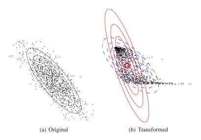
**Figure 3.6:** Illustration of linearization based (EKF) approximation to the transformation in Figure 3.5. The Gaussian approximation is formed by calculating the curvature at the mean, which results in bad approximation further from the mean. The true distribution is presented by the blue dotted line and the red solid line is the approximation.
