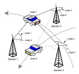
**Figure 1.3:** In multiple target target tracking the data association problem has to be solved, which means that it is impossible to know without any additional information, which target produced which measurement.
