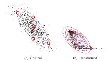
**Figure 3.7:** Illustration of unscented transform based (UKF) approximation to the transformation in Figure 3.5. The Gaussian approximation is formed by propagating the sigma points through the non-linearity and the mean and covariance are estimated from the transformed sigma points. The true distribution is presented by the blue dotted line and the red solid line is the approximation.
