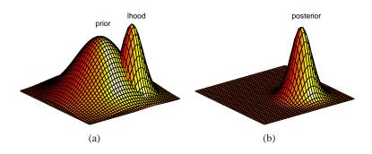
**Figure 3.2:** Visualization of the update step: (a) Prior distribution from prediction and the likelihood of measurement just before the update step. (b) The posterior distribution after combining the prior and likelihood by Bayes' rule.
