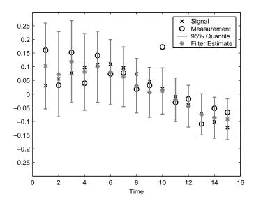
**Figure 1.7:** The result of computing the filtering distributions for the discrete-time resonator model. The *estimates* are the posterior means of the filtering distributions and the quantiles are the 95% quantiles of the filtering distributions.
