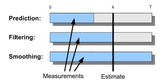
**Figure 1.6:** State estimation problems can be divided into optimal prediction, filtering and smoothing depending on the time span of measurements available with respect to the estimated state time span.
