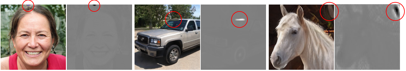
Figure 1. Instance normalization causes water droplet -like artifacts in StyleGAN images. These are not always obvious in the generated images, but if we look at the activations inside the generator network, the problem is always there, in all feature maps starting from the 64 \times 64 resolution. It is a systemic problem that plagues all StyleGAN images.
