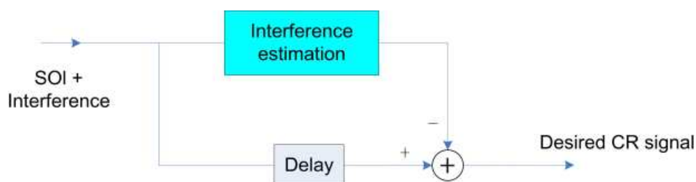
FIGURE 4.1: Block diagram of a CR receiver using interference estimation and cancellation.
