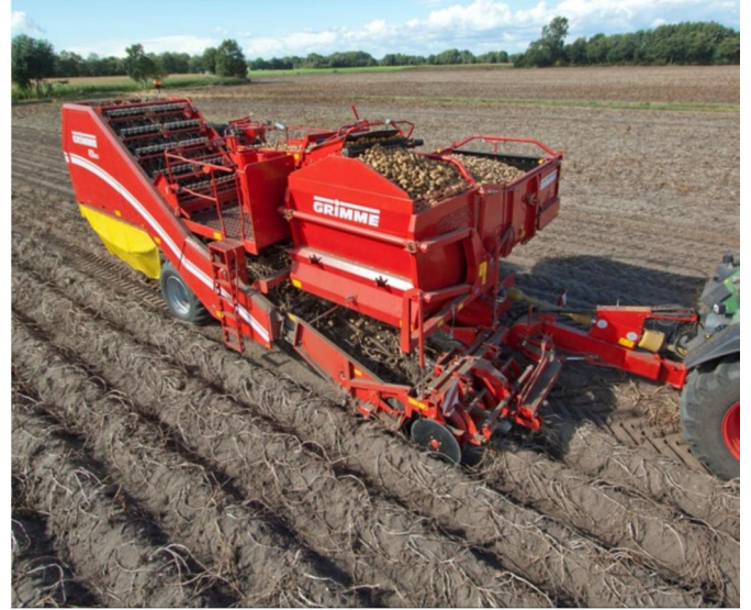
Figure 4. Potato harvester with drawbar steering and steerable rear wheels.
