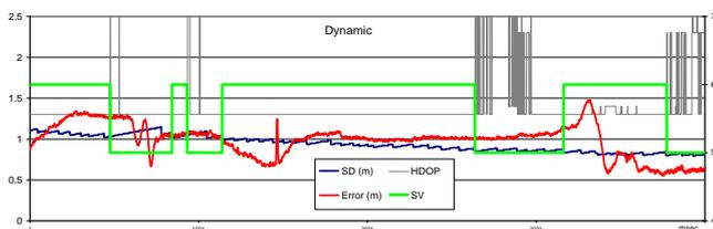
Figure 1. HDOP, the number of SVs and the accuracy.
