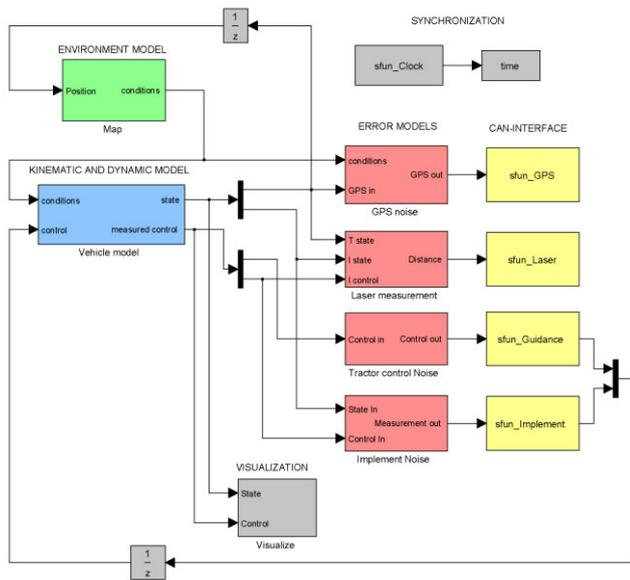
Figure 3. The overall structure of the simulator in Matlab Simulink - environment.
