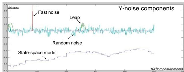
Figure 5. Y-axis errors caused by different components.
