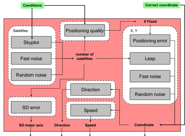
Figure 4. The structure of the GPS-noise model
