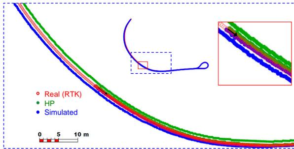
Figure 7. The recorded trajectory of the real vehicle and the simulated trajectory with the same control values.
