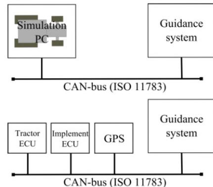
Figure 2. The simulation environment and the real system
