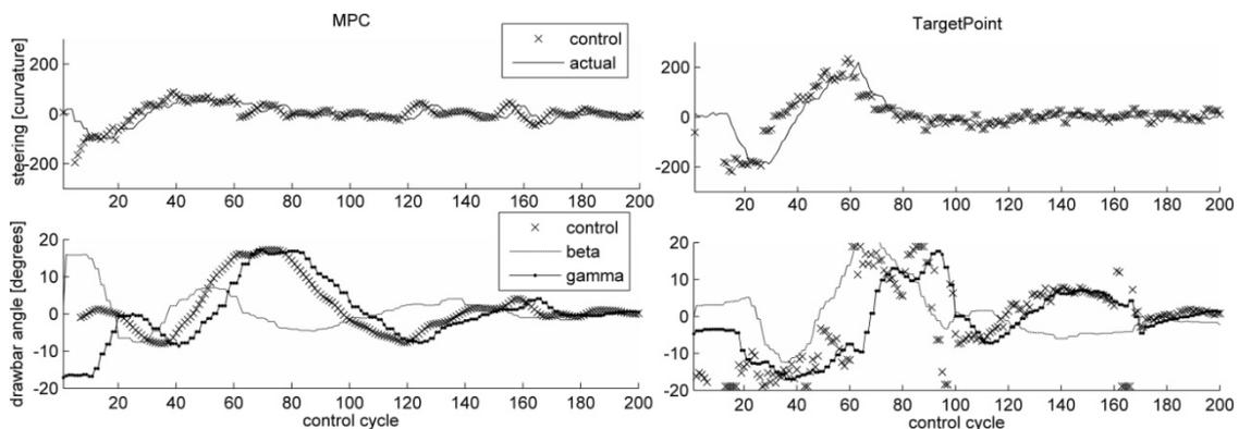
**Figure 4 Control values of steering and joint angles using MPC and Target Point –algorithms in step response test.**
