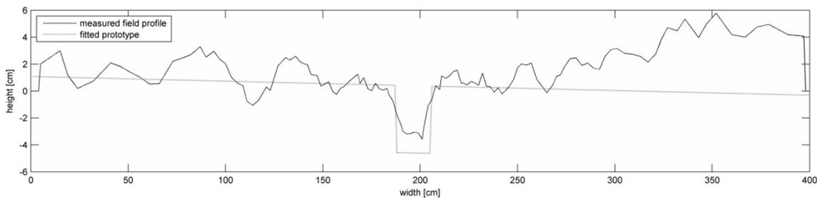
Figure 3 Laser scanner measurements and fitted mark prototype, note that the scales of x- and y-axis are different.
