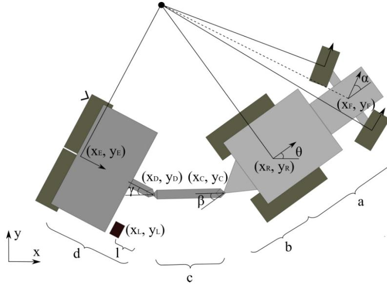
Figure 2 Variables and parameters of the kinematic model.
