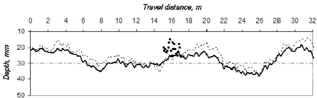
Figure 6. Seeding depth estimated by model (solid) and measured by hand (square) at a seeding depth of 30 mm. Dot line is the seeding depth estimated by the model using 5<sup>th</sup> coulter's measurements.
