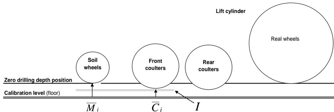
Figure 2. Position of measurement wheels and coulters from the calibration level, and model parameters.  $M$  is distance from the soil wheel to the calibration level,  $C$  distance from the coulters to the calibration level, and  $I$  is the inclination correction factor.
