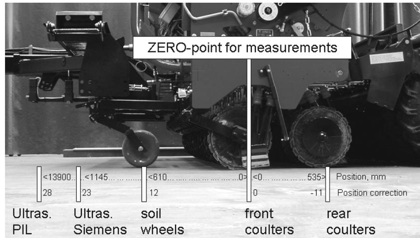
Figure 1. Position of sensors used in the depth control and measurement system of the drill.
