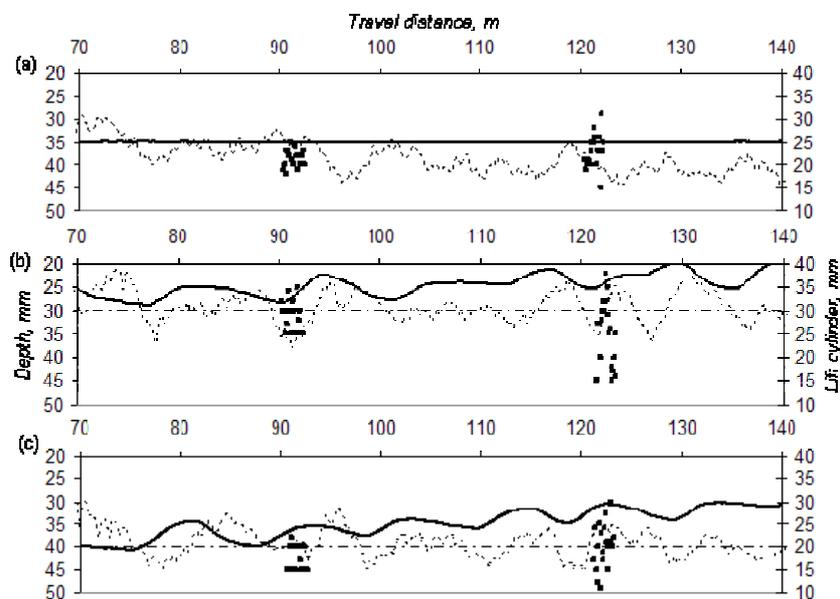
Figure 5. Results of test for the control system, (a) results of the manual test run, (b) and (c) results from test runs 30 mm and 40 mm. Solid line describes position of the lift cylinder. Dot lines describe working depth estimated by the model. Square plots represent real depths of seeds.
