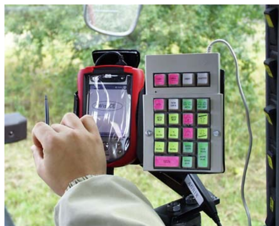
Fig. 3. The HMI implemented with standard PDA and external keyboard.
