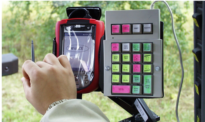
Figure 4. The HMI implemented with standard PDA and external keyboard.
