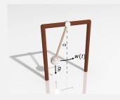
Pendulum with mass m = 1, pole length L = 1 and random force w(t):
