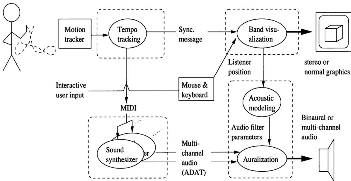
**FIGURE 1.** The Virtual Orchestra components. The tempo tracking module sends synchronization signal to the animation (visualization) module and MIDI signals to sound synthesis modules. The other user can control the viewpoint of a virtual concert hall with mouse and keyboard.
