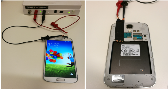
Fig. 25. Power measurement setup.
